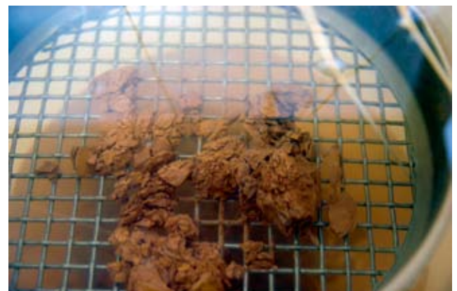
3 Tonagglomerat während des Zerfallstests Clay agglomerate during a disintegration test
