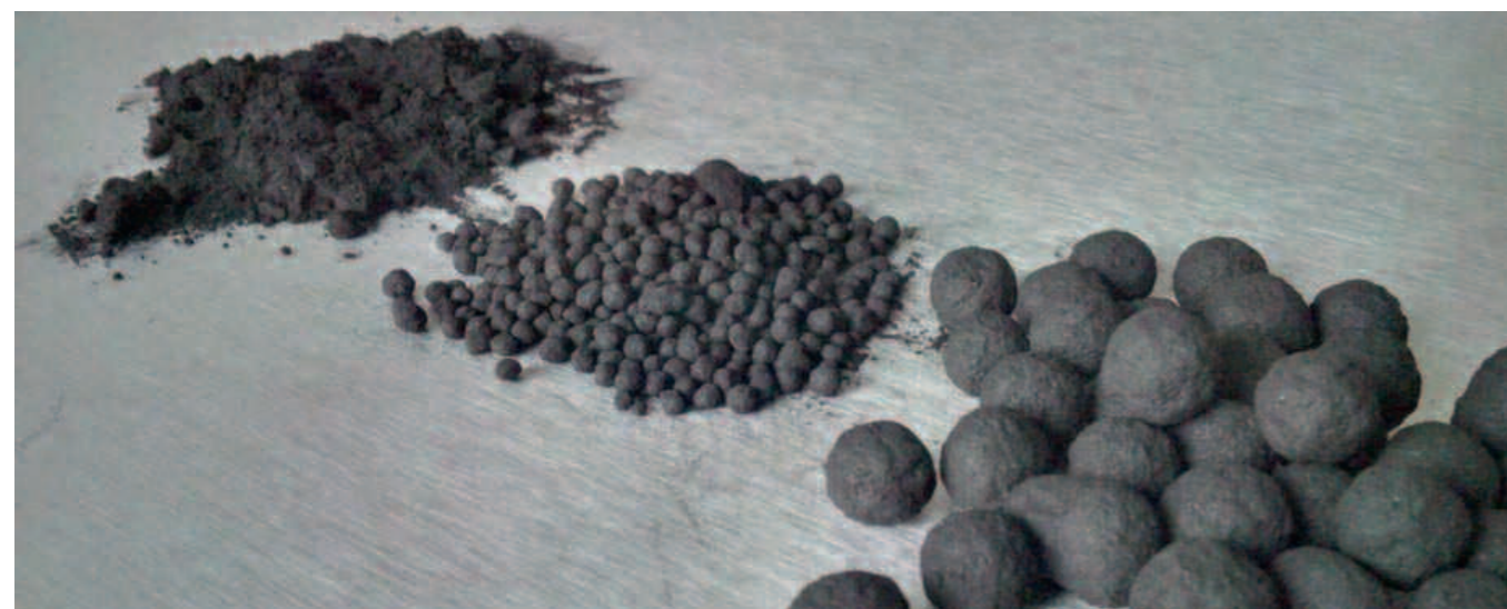
2 Kohlegranulation (v.l.n.r. Staub, kleine Granulate, große Granulate) Coal granulation (left to right: dust, small-size granulate, large-size granulate)
